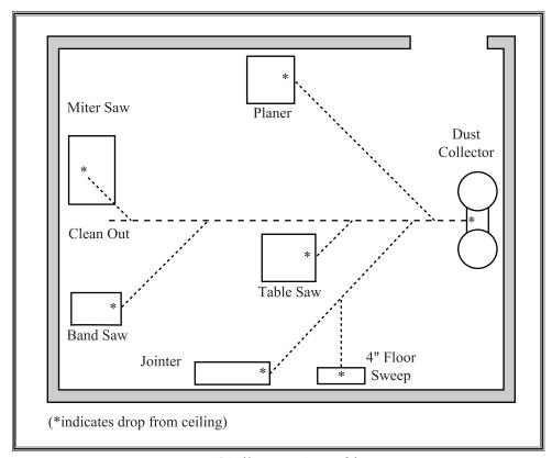
Figure 23. Bird's eye view of layout.
